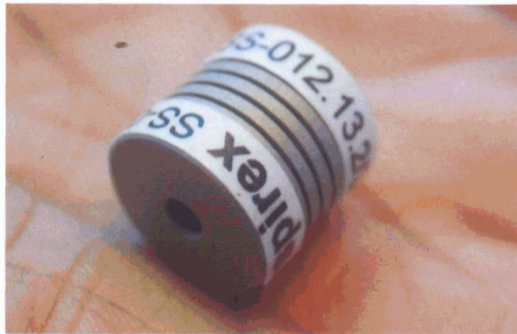
Spirex encoder coupling with 3 mm bore
