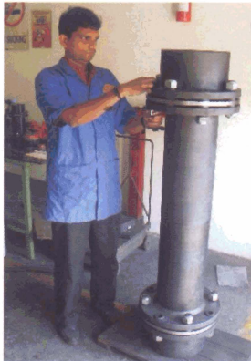
flexiMax membrane coupling with a rating of 28000 Nm for hot strip mill in a steel plant.
