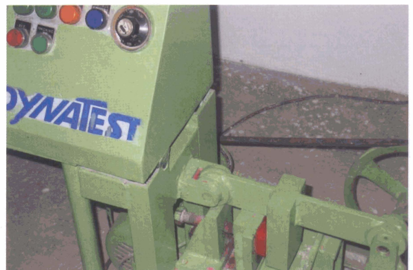
TorTest - Test Bed for measurement of Torque and stiffness characteristics.
