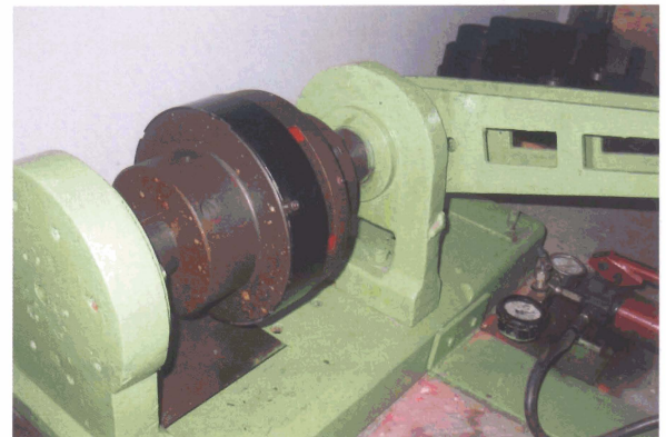
TorTest - Test Bed for measurement of Torque and stiffness characteristics.
